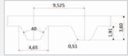
L TİPİ KAYIŞ PROFİLİ L TYPE BELT PROFILE
